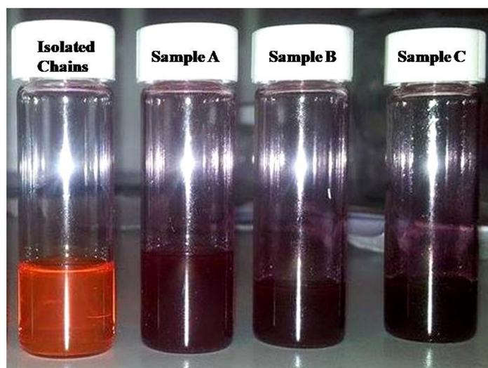
**Figure 1** Photographs of a fully dissolved P3HT solution prepared in 3-HT, aggregated solutions prepared from THF (sample A),  $\text{CHCl}_3$  (sample B) and Toluene (sample C).
