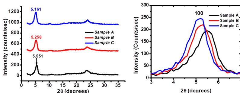
**Figure 3** Wide-angle X-ray diffraction pattern of nanostructured P3HT films deposited on silicon. The diffractograms shows strongly enhanced 100 reflections Bragg peak yielding a form 1 monoclinic crystal structure. The 100 Bragg peak increases intensity from sample A to C with reduced full wave at half maximum (FWHM)
