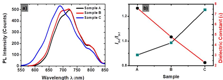
**Figure 8** The PL spectra collected from sample A, B and C (a) and the graph showing increasing  $I_{0,0}/I_{0,1}$  intensity ratios in PL with decreasing solvent dielectric constants
