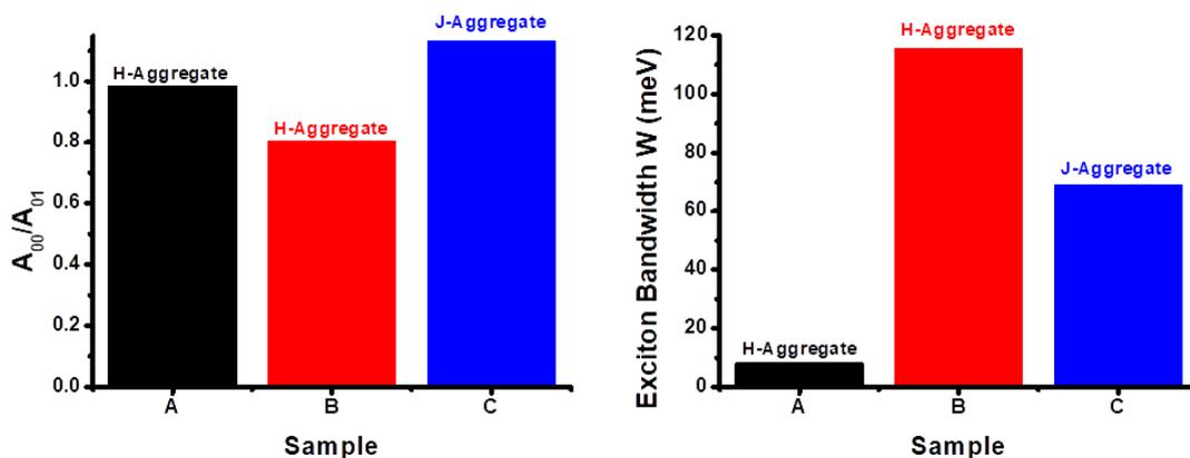
**Figure 7** The absorption intensity ratios  $A_{0,0}/A_{0,1}$  and the excitonic band widths for three samples A, B, C
