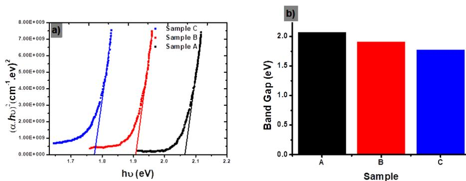
**Figure 10** A graph of  $(\alpha h\nu)^2$  versus photon energy ( $h\nu$ ) for P3HT crystals (a) and a bar graph showing decreasing band gap energy of P3HT crystals with the solvent used for fabrication (b).
