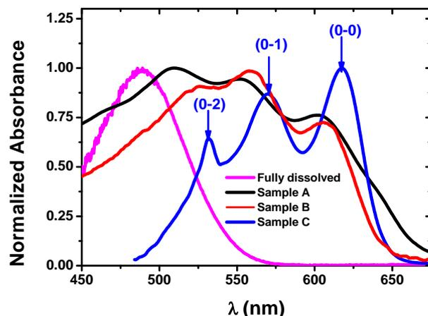
**Figure 6** The typical absorption spectra from isolated chains P3HT 3-HT, thin films prepared from THF (sample A), in  $\text{CH}_2\text{Cl}_2$  (Sample B) and in toluene (sample C). The vibronic features of the P3HT aggregates and fibers are labeled according to the number of vibrational quanta in the excited state
