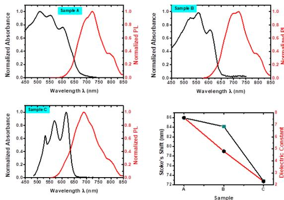
**Figure 9** The absorption and the PL spectra collected from sample A, B and C showing decrease in Stoke's shift with decreasing solvent polarities
