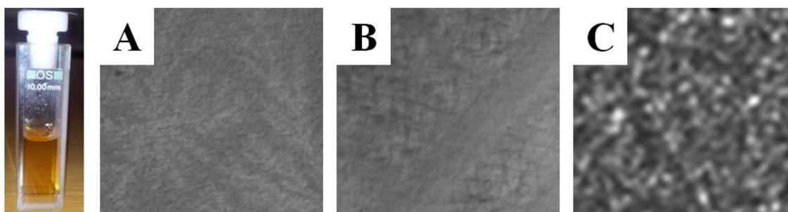
**Figure 2** Diagram showing a fully dissolved P3HT solution in a 10.0 mm cuvette prepared from 3-HT and thin films of P3HT solutions prepared from THF (sample A),  $\text{CHCl}_3$  (sample B) and Toluene (sample C). (The micrograph sizes are 250  $\mu\text{m}$  by 250  $\mu\text{m}$ )
