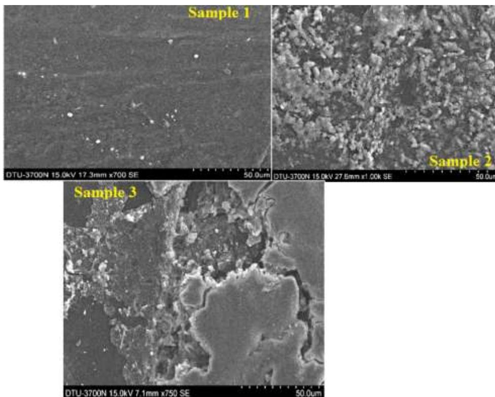
**Figure 4** SEM micrograph of samples 1, 2 &3 after 40 days of water absorption test.
