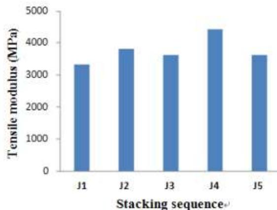
**Fig. 3** Variation of Tensile modulus (TM) with stacking sequence of jute-polyester composites
