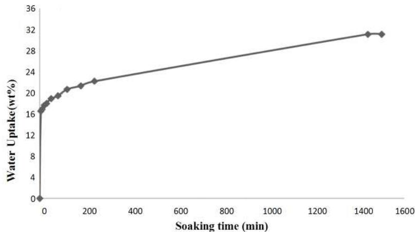
**Fig. 7** Water uptake (%) of jute-polyester composites
