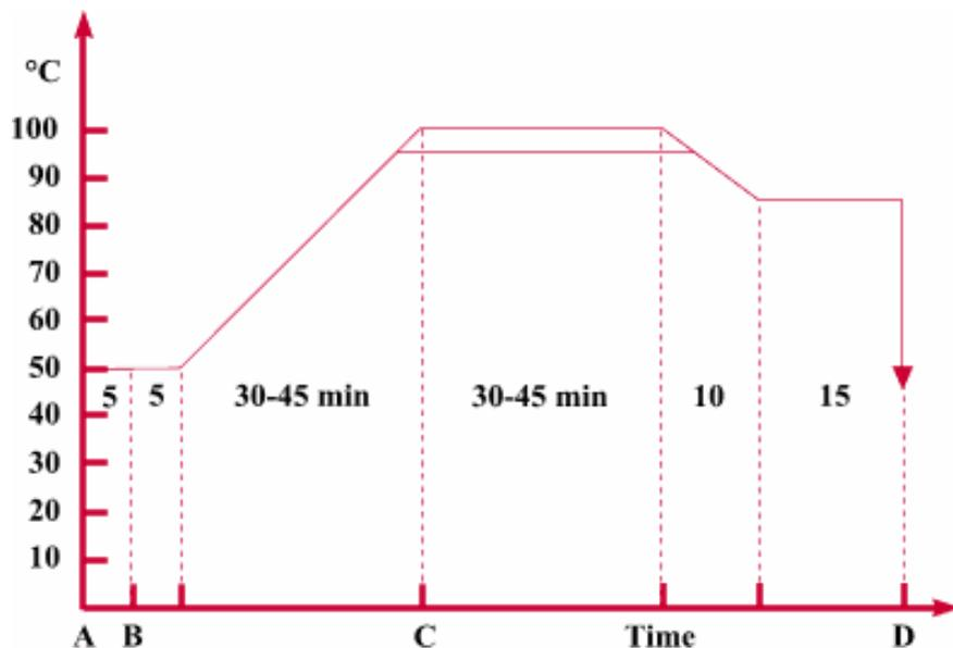
**Figure 1** Dyeing curve with conventional reactive dyes with exhaust method
