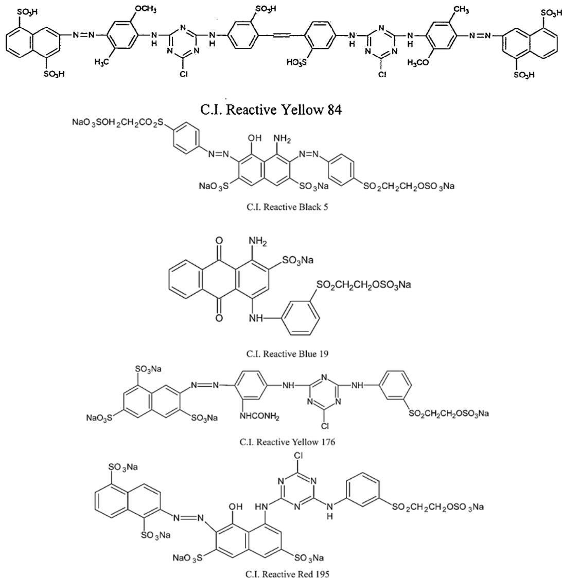
**Figure 2** Chemical Structure of conventional reactive dyes
