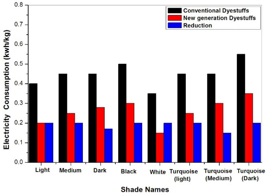
**Figure 5** Electricity consumption reduction analysis and new generation dyestuffs
