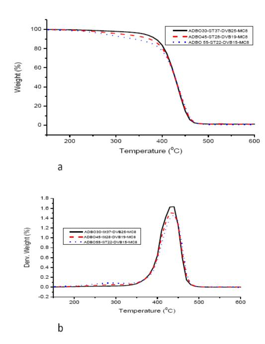
**Figure 8** (a) TGA curves of ADBO polymer with increasing ADBO concentration; (b) TGA derivative curves of ADBO polymers with increasing ADBO concentration.
