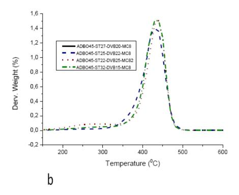
**Figure 9** (a) TGA curves of ADBO polymers with increasing DVB concentration; (b) TGA derivative curves of ADBO polymers with increasing DVB concentration.
