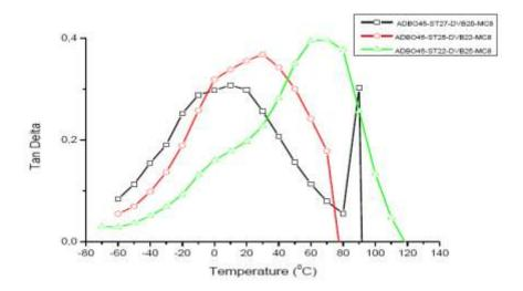
**Figure 6** Temperature dependence of the loss factor,  $\tan \delta$  of ADBO polymers prepared by varying the DVB concentration while the content of ST plus DVB remained constant at 47%
