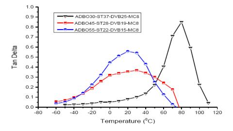
Figure 4 Temperature dependence of the loss factor,  $\tan \delta$  of ADBO polymers prepared by varying the ADBO concentration while ratio of ST: DVB remained constant at 3:2
