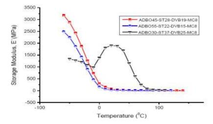
**Figure 2** Temperature dependence of the storage modulus of ADBO polymers prepared by varying the ADBO concentration while ratio of ST: DVB remained constant at 3:2
