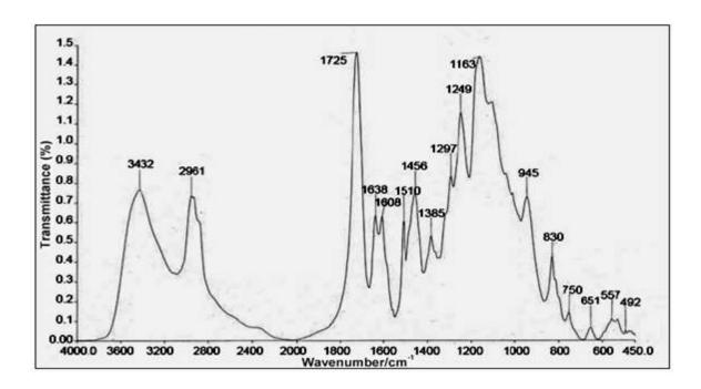
Figure 1 FTIR spectrum of ESOA-BisGMA blend (50:50 wt%)
