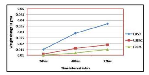
Figure 7 Corrosion test of EB<sub>50</sub>, UJEBC and HJEBC
