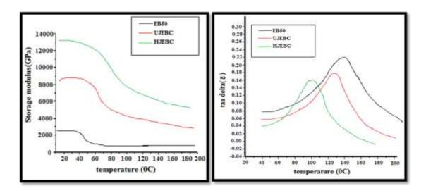
**Figure 6** (a) Storage modulus (b)  $\tan \delta$  of EB<sub>50</sub>, UJEBC and HJEBC
