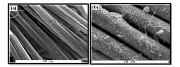
Figure 2 SEM of (a) Untreated jute fiber (b) HEA treated jute fiber
