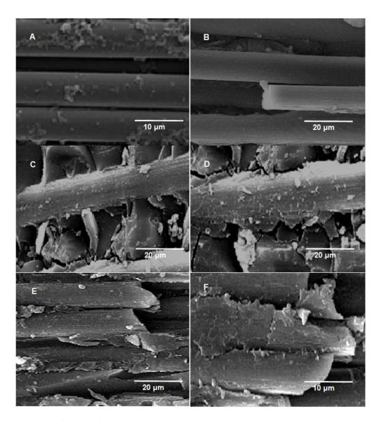
**Figure 1** Fractographic images of (A) PCL-CFs-NDs at 10  $\mu$ m; (B) Epoxy/PCL-CFs-NDs 1 at 20  $\mu$ m; (C) Epoxy/PCL-CFs-NDs 3 at 20  $\mu$ m; (D) Epoxy/PCL-CFs-NDs 5 at 20  $\mu$ m; (E) Epoxy/PCL-CFs-NDs 10 at 20  $\mu$ m; and (F) Epoxy/PCL-CFs-NDs 10 at 10  $\mu$ m.
