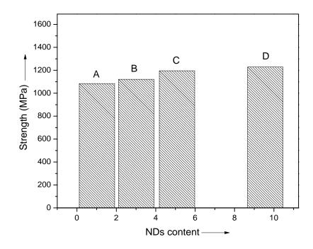
**Figure 3** Tensile strength of composite specimens having carbon fibers with different NDs content (A) Epoxy/PCL-CFs-NDs 1; (B) Epoxy/PCL-CFs-NDs 3; (C) Epoxy/PCL-CFs-NDs 5; and (D) Epoxy/PCL-CFs-NDs 10.
