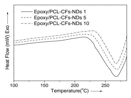
Figure 2 DSC melting curves of Epoxy/PCL-CFs-NDs composites.
