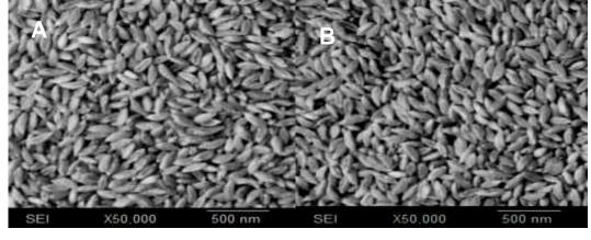
Fig. 3 SEM micrographs of (A) PEEA/PMA/Zein 1; and (B) PEEA/PMA/Zein 5.
