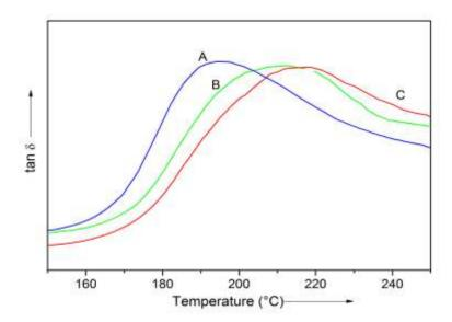
**Fig. 6** Plots of tanδ vs. temperature for (A) PEEA/PMA blend; (B) PEEA/PMA/Zein 1; and (C) PEEA/PMA/Zein 5 nanocomposite.
