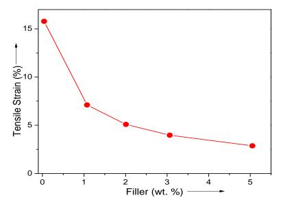
Fig. 5 Tensile strain of PEEA/PMA blend with zein loading.
