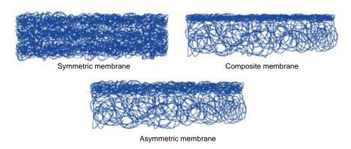
Figure 5 Schematic representation of basic membrane structures.
