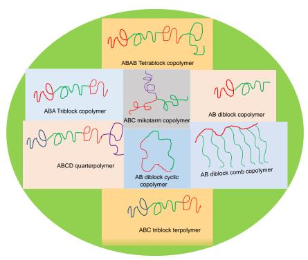
**Figure 2** Block copolymer architechture; AB diblockcopolymer; ABC triblockterpolymer; ABA triblockcopolymer; ABAB tetrablockcopolymer; ABCD quarterpolymer; ABC mikotarmstar copolymer; AB diblockcomb copolymer; AB diblockcyclic copolymer.
