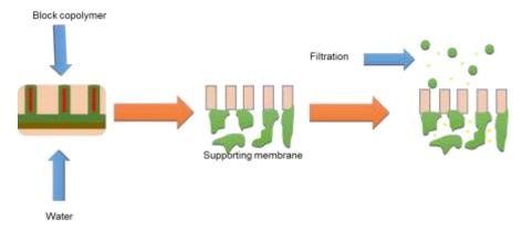
Figure 6 Illustration of the composite membrane formation.
