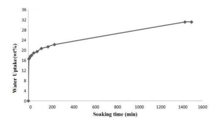
Fig. 7 Water uptake (%) of jute-polyester composites
