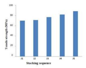
Fig. 2 Variation of Tensile strength (TS) with stacking sequence of jute-polyester composites
